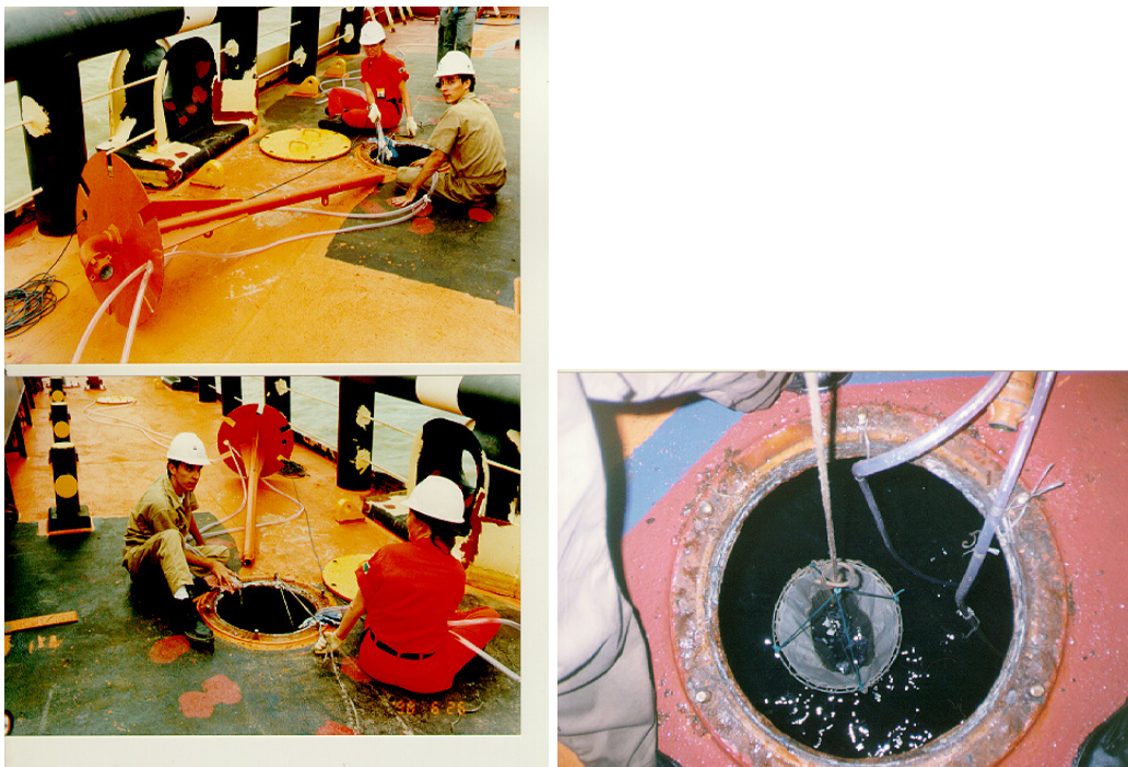
Figure 17: Sampling ballast water during an experiment in NT Lavras (Photos: Petrobras).
