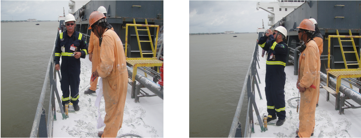
Figure 19: Port State Control Officer and ship's crew sampling ballast water through the sounding pipe to verify its salinity with a portable refractometer (CPRJ/MB) 79 .
