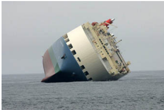
Figure 16: Photo of the M/V Cougar-Ace that while exchanging ballast at sea tumbled but didn't sink on a voyage between Japan and U.S and Canada west coast ports and which became a classical image regarding to safety operational aspects during the BWE. 42
