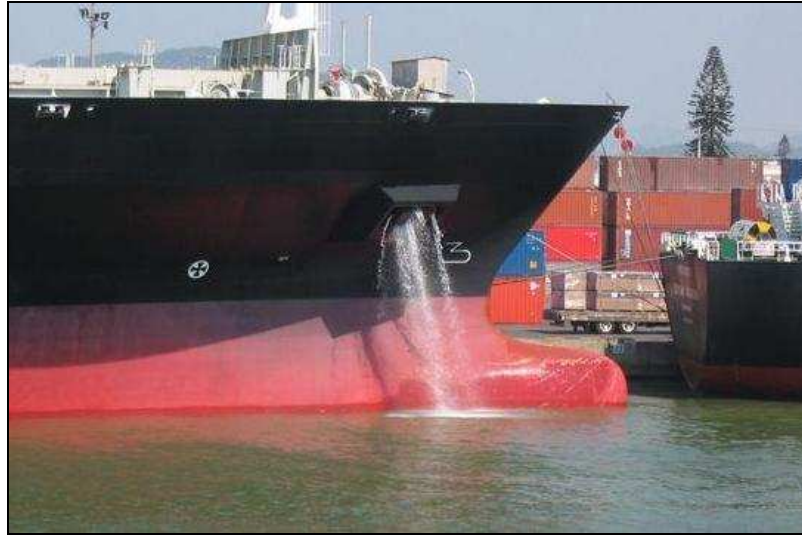
Figure 1. Ship discharging ballast water 5
